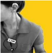
The Beetle is a lightweight Bluetooth headset that transmits speech directly from your cell phone to your hearing aid. Simply switch the hearing aid to telecoil, place the ear hook behind the ear, and clip the small Bluetooth receiver to your lapel. The phone will ring through the hearing aid and can be answered by pressing a button. The Beetle is rechargeable and allows for 6 hours talk time.
